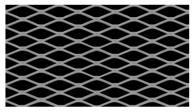
LW Pitch:30.48mmStrand Width:2.36mmSW Pitch:11.72mmThickness:1.50mmWeight:5.06 kg / m2Open Area:59%
